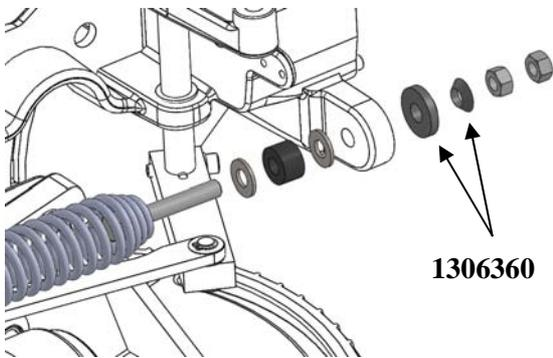
**Tighten the spring (with the help of a crank (spanner) for example) bearing in mind that the tighter the screw, the speed of the clay is increased. Once the correct tension has been obtained, tighten the locknut.**
