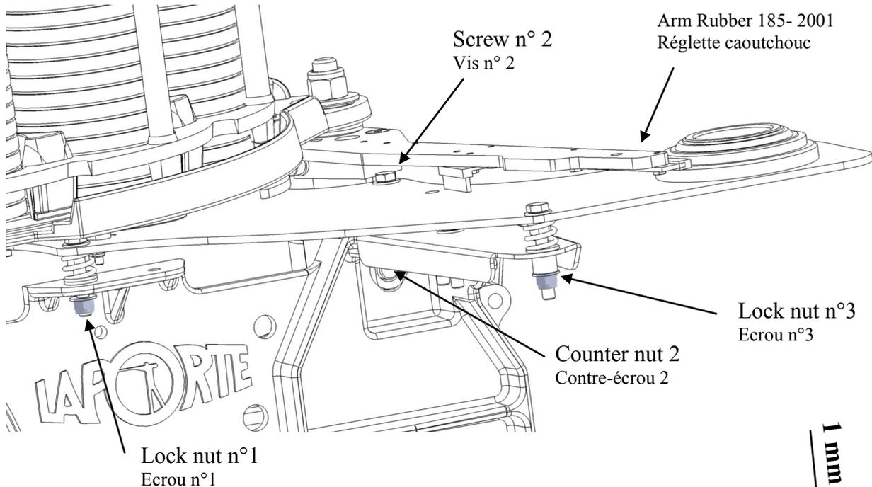
1 -Use the adjustment screw to raise or lower the throwing plate in order to obtain a space of around 1mm between the clay and the arm rubber.
