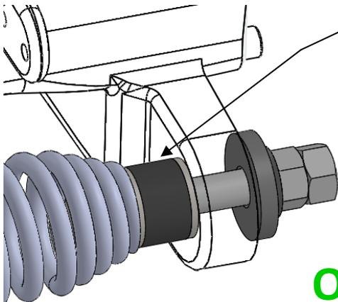
**Adjust the tension of the spring by tightening the nut at the back of the machine.**
