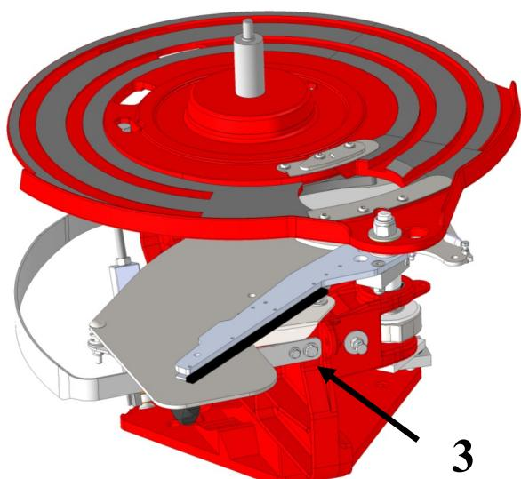
**Fixing the safety guard to the front of the machine.**
