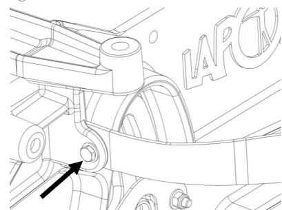
**Fixing the safety guard to the rear of the machine.**
