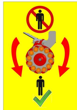
It is essential to access the machine from behind! Only one person should have access to the machine when it is being used. It is recommended to build sheltering walls to avoid broken clays or debris flying around. The user should always wear protection glasses to avoid eye injury from flying broken clays.
