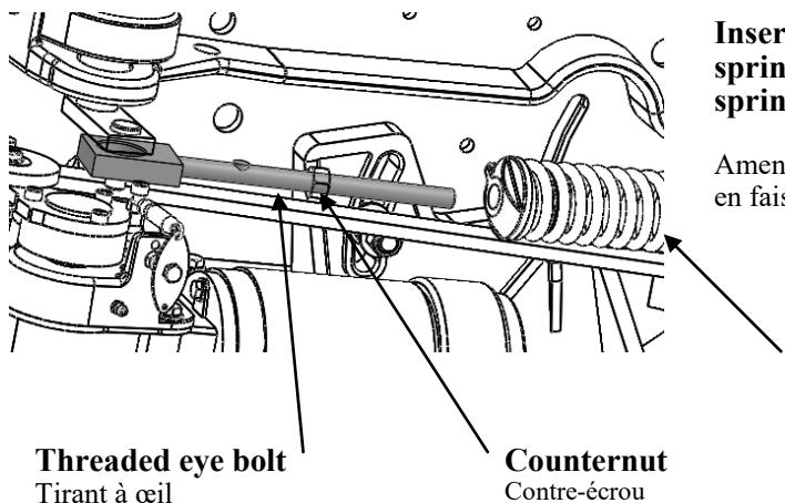
Insert the threaded eye bolt into the front of the spring by turning the throwing arm, tighten the spring by hand.
