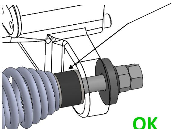
The silent rubber block should be tightened without being compressed.
