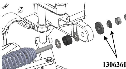
Tighten the spring (with the help of a crank (spanner) for example) bearing in mind that the tighter the screw, the speed of the clay is increased. Once the correct tension has been obtained, tighten the locknut.
