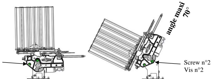
1– Check that the screw of rotation n° 1 is not completely blocked, if it is the case it is necessary to loosen it.
