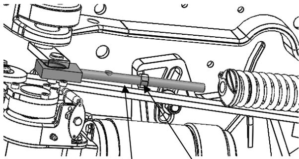
**Insert the threaded eye bolt into the front of the spring by turning the throwing arm, tighten the spring by hand.**
