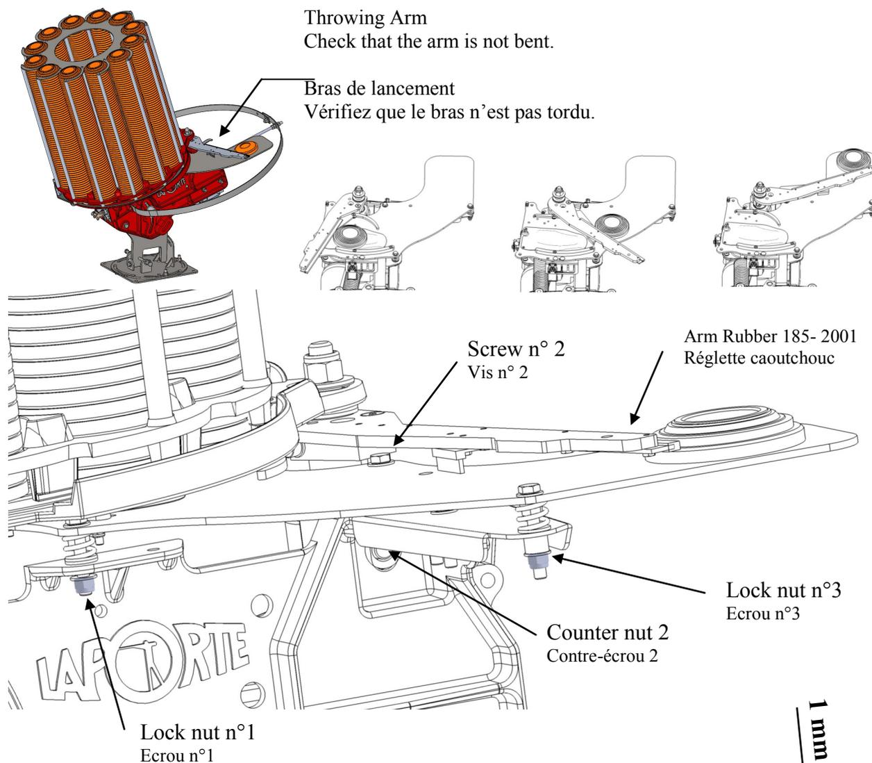
1 -Use the adjustment screw to raise or lower the throwing plate in order to obtain a space of around 1mm between the clay and the arm rubber.
